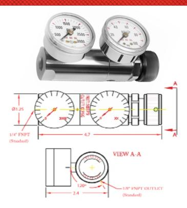
This miniature, two stage (1st stage piston sensed & 2nd stage Elgiloy® diaphragm sensed) regulator, is intended for high purity, low-flow gas services, regulating a broad range of media compatible with materials of construction.
