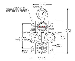
All dimensions are reference & nominal Metric [millimeter] equivalents are in brackets
