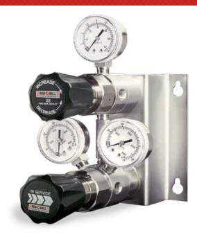
The CS-2200 Series is a complete high purity changeover system which combines the changeover regulator and a line regulator into a compact wall mount system for specialty, corrosive, and pyrophoric gases.
